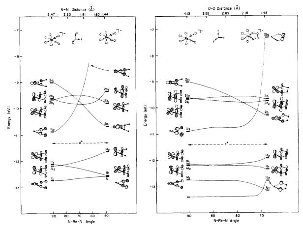
Figure 5. Walsh diagram for the coupling of two NO ligands in  $[ReCl_4(NO)_2]^-$ : (a) involving the formation of a N-N bond; (b) involving the formation of an O-O bond.
