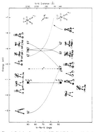
Figure 4. Evolution of energy levels of [ReCl<sub>4</sub>(NS)<sub>2</sub>]<sup>-</sup> along an idealized reaction coordinate, forming a N-N bond. Note the N-Re-N angle scale at the bottom and the nonlinear N-N distance scale at the top.
