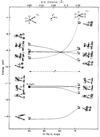
Figure 2. Evolution of energy levels of  $[ReCl_4(NS)_2]^-$  along an idealized reaction coordinate, forming a S-S bond. Note the N-Re-N angle scale at the bottom and the nonlinear S-S distance scale at the top.
