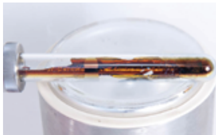
Shown here in its liquid form, tetraamminelithium ( Li(NH_3)_4 ) is unusual because of its low freezing point, nearly 150 degrees Celsius below that of any other metal. (Photograph courtesy of Matthew Lodge.)
