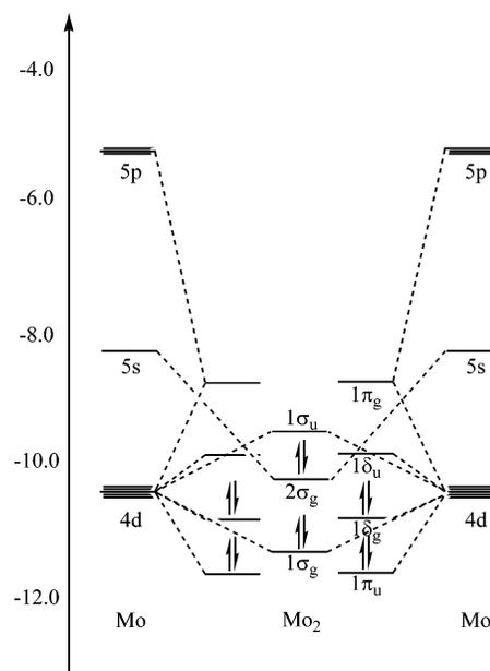
**Figure 1.** Orbital interaction diagram showing the valence energy levels for Mo and Mo<sub>2</sub>. The energy levels come from an extended Hückel calculation.
