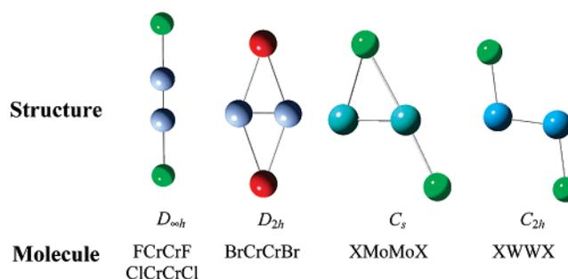
**Figure 7.** Pictorial summary of the global minima for XMMX molecules. Where X is not specified, that geometry is the minimum energy isomer for all three  $X = F, Cl,$  and  $Br$ . Geometrical parameters for all the optimized isomers are given in Table 1.
