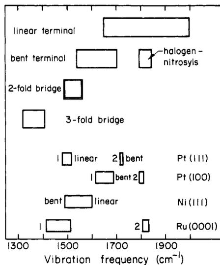
**Figure 1.** NO stretching frequencies of nitrosyls of known structure, following Pirug et al., and of adsorbed NO. The numbers 1 and 3 refer to the sequence in which the species appear on the surface as a function of exposure. This figure is taken from Figure 6.12 of ref 9. (Reprinted with permission from ref 9. Copyright 1982, Academic Press.)
