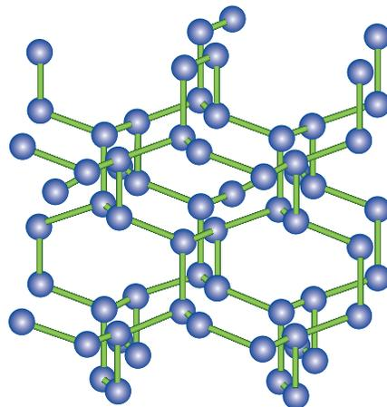
The shape of a nitrogen molecule depends on pressure. At a pressure of more than 110 Gigapascals and a temperature of 2,000 kelvins, the molecules transform into a three-dimensional polymeric network.
