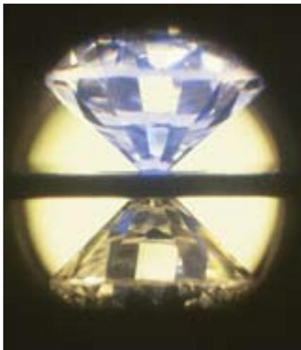
In order to generate pressures similar to those found at the center of the Earth, researchers use diamonds as anvils. The high-pressure “cell” is created by a bagel-shaped gasket that encloses a reaction space of roughly 1 cubic millimeter. Image is courtesy of Dr. Russell Hemley, Carnegie Institution of Washington.
