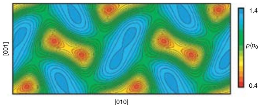
A computer simulation predicts that at higher pressures, metallic lithium moves away from a traditional close-packed arrangement. This image shows the calculated electron density of the 2s orbitals of lithium. Atoms of lithium, located in the regions of lowest 2s electron density (orange spots), pair up, whereas electron density moves into the crevices between atom pairs (blue).
